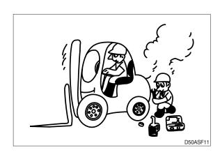
Always remember that the hydraulic oil circuit is under pressure. When feeding or draining the oil or carrying out inspection and maintenance, release the pressure first.
